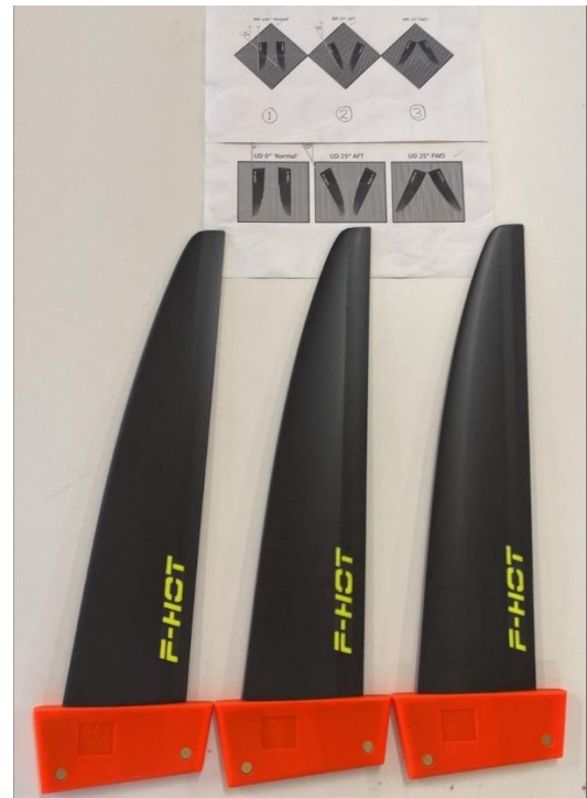
Figure 2: Nominal, Wash-in and Wash-out 44 cm span fins
