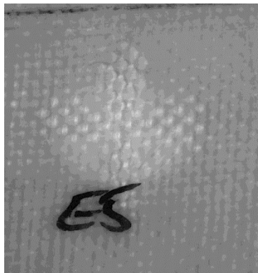
Fig. 5. Front face code 3: cross delamination.
