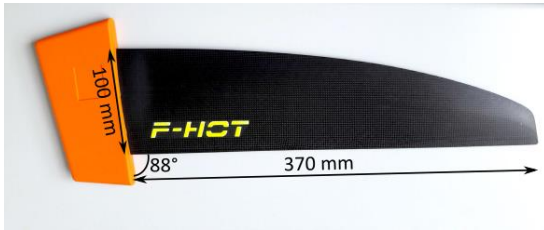
Figure 1 Slalom fin geometry
