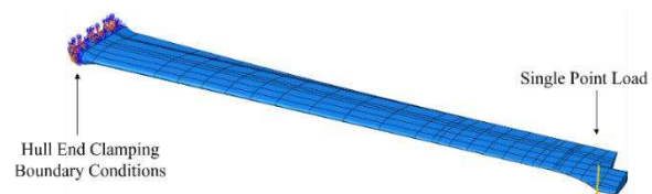
Figure 15 FEA validation setup.
