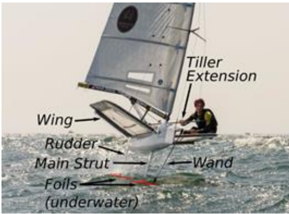
Figure 3 Parts of a foiling moth © Rui Brites (adapted)
