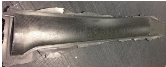
Figure 9 Main strut on removal from the mould.
