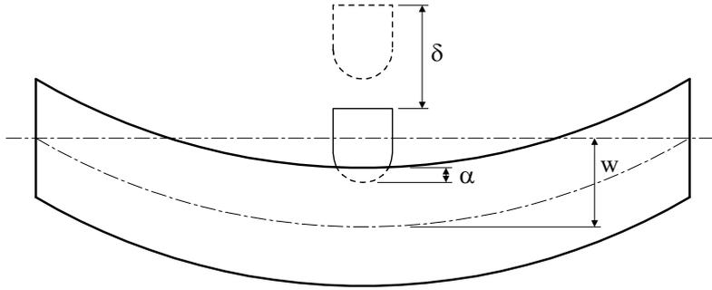
Fig. 1. Impact Force ( $P$ ), Displacement ( $\delta$ ), Indentation ( $\alpha$ ) and Deflection ( $w$ ).
