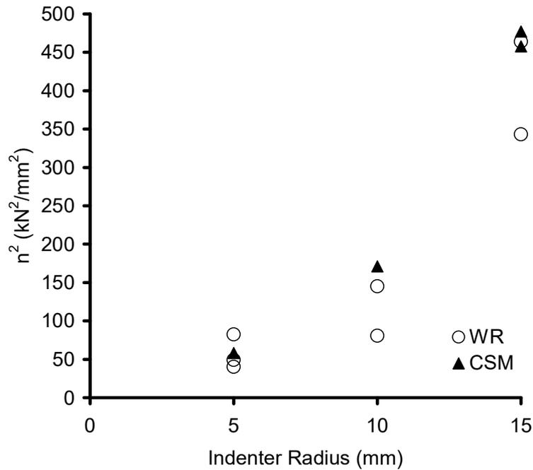
Fig. 9. Power law coefficient 'n' vs. indenter radius.
