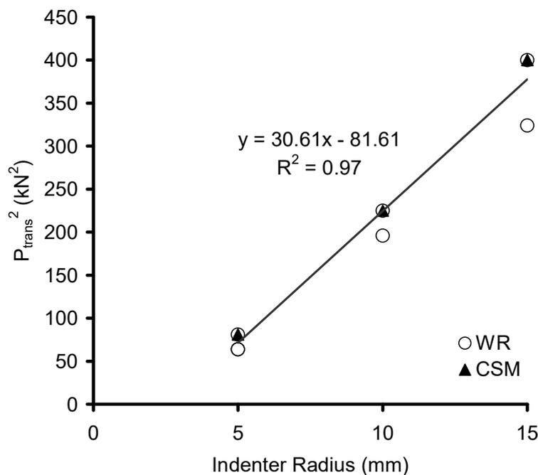
Fig. 10. Transition to linear contact response.
