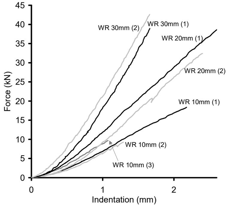
Fig. 6. Woven roving averaged contact responses.
