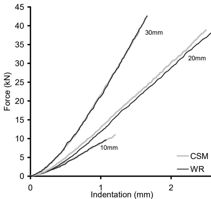
Fig. 8. Comparison of stiffest WR and CSM contact responses.
