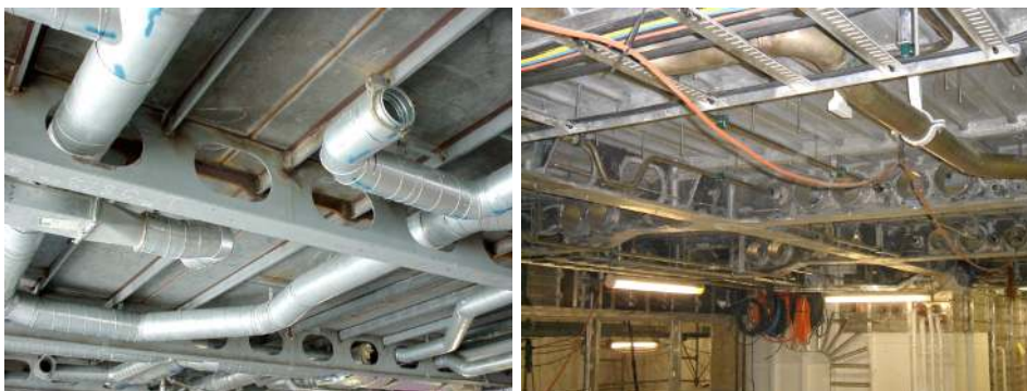
Figure 15: Typical ‘tween deck depths for service runs (images courtesy of BMT Nigel Gee).
