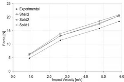
**Figure 16:** Maximum force vs. impact velocity. Thick (5.92 mm) circular plates.
