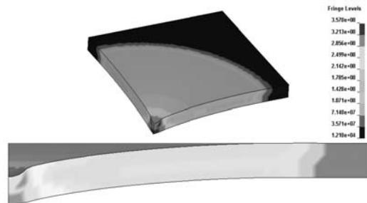
**Figure 20:** Maximum effective stress distribution. Thick (5.92 mm) circular plates, impact velocity 5.85 m/s.
