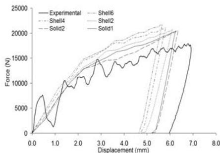
**Figure 10:** Force-displacement curves. Thick (5.92 mm) circular plates, impact velocity 5.85 m/s.
