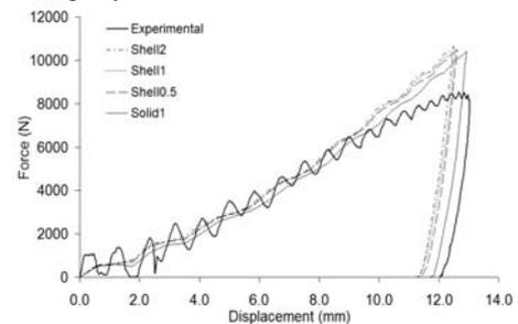
**Figure 12:** Force-displacement curves. Thin (2.00 mm) circular plates, impact velocity 5.90 m/s.
