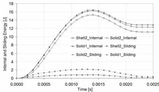
**Figure 21:** Internal and sliding energy dissipation. Thick (5.92 mm) circular plates, impact velocity 2.61 m/s.
