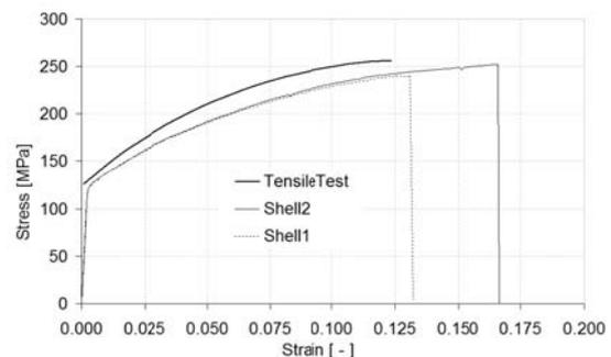
**Figure 9:** Numerical and experimental engineering stress-strain curves. Thickness 2.00 mm.
