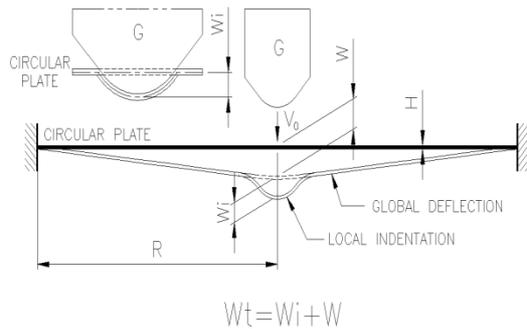
**Figure 1:** Clamped circular plate struck transversely at the centre by a mass.
