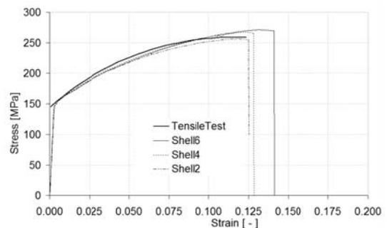
**Figure 8:** Numerical and experimental engineering stress-strain curves. Thickness 5.92 mm.
