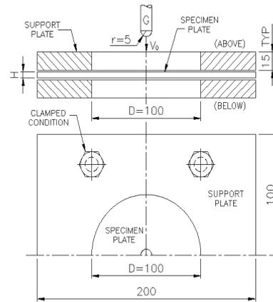
**Figure 2:** Circular plate specimen in clamped condition (dimensions in millimetres).
