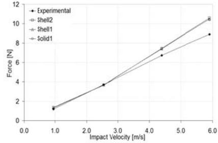
**Figure 18:** Maximum force vs. impact velocity. Thin (2.00 mm) circular plates.
