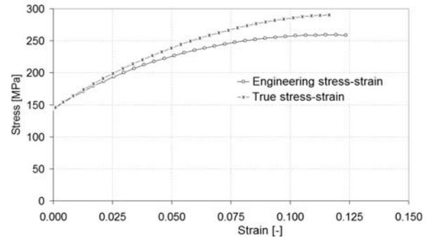
**Figure 5:** Engineering and true stress-strain curves (experimental). Thickness 5.92 mm.
