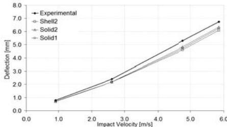
**Figure 15:** Maximum deflection vs. impact velocity. Thick (5.92 mm) circular plates.
