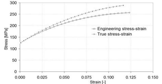
**Figure 6:** Engineering and true stress-strain curves (experimental). Thickness 2.00 mm.
