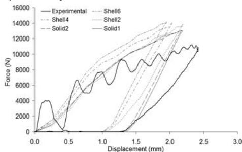
**Figure 11:** Force-displacement curves. Thick (5.92 mm) circular plates, impact velocity 2.62 m/s.
