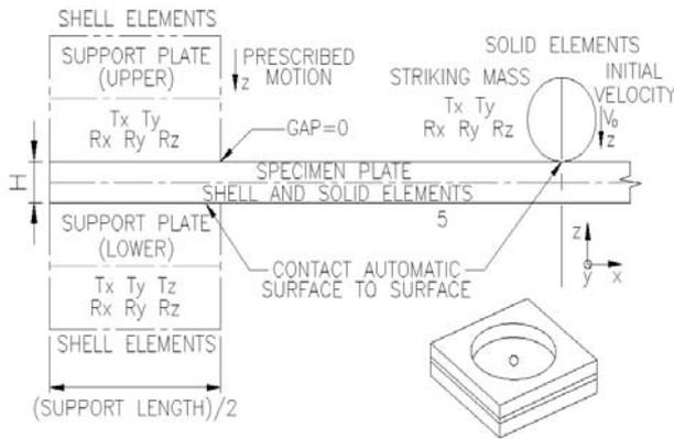
Figure 3: Details of finite element model.
