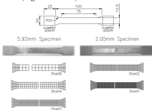
**Figure 7:** Tensile test specimens and their numerical simulation.
