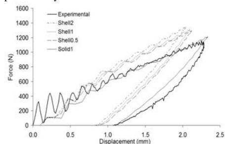
**Figure 13:** Force-displacement curves. Thin (2.00 mm) circular plates, impact velocity 0.95 m/s.
