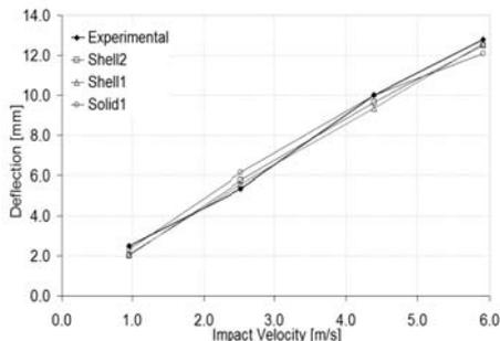
**Figure 17:** Maximum deflection vs. impact velocity. Thin (2.00 mm) circular plates.
